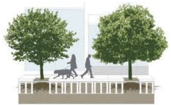
Cross section of Silva Cells
